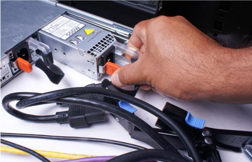
Figure 9. Replacing the outer power supply
