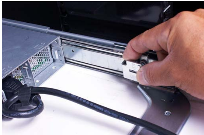
Figure 4. Attaching the inner CMA attachment bracket
