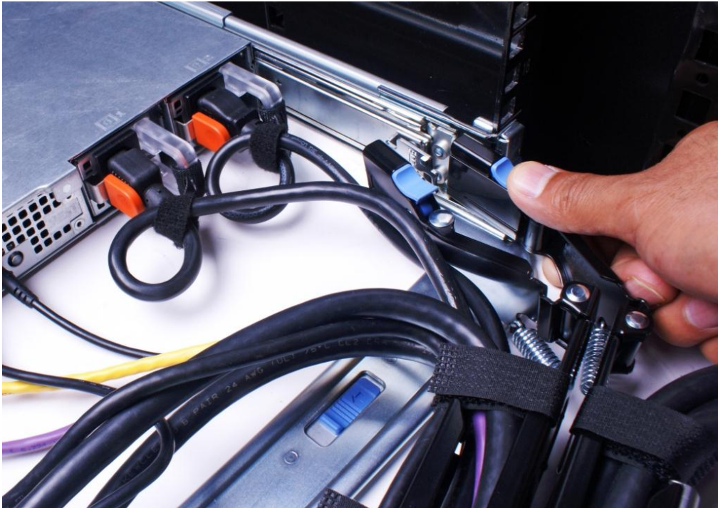
Figure 8. Disconnecting the CMA attachment housings
